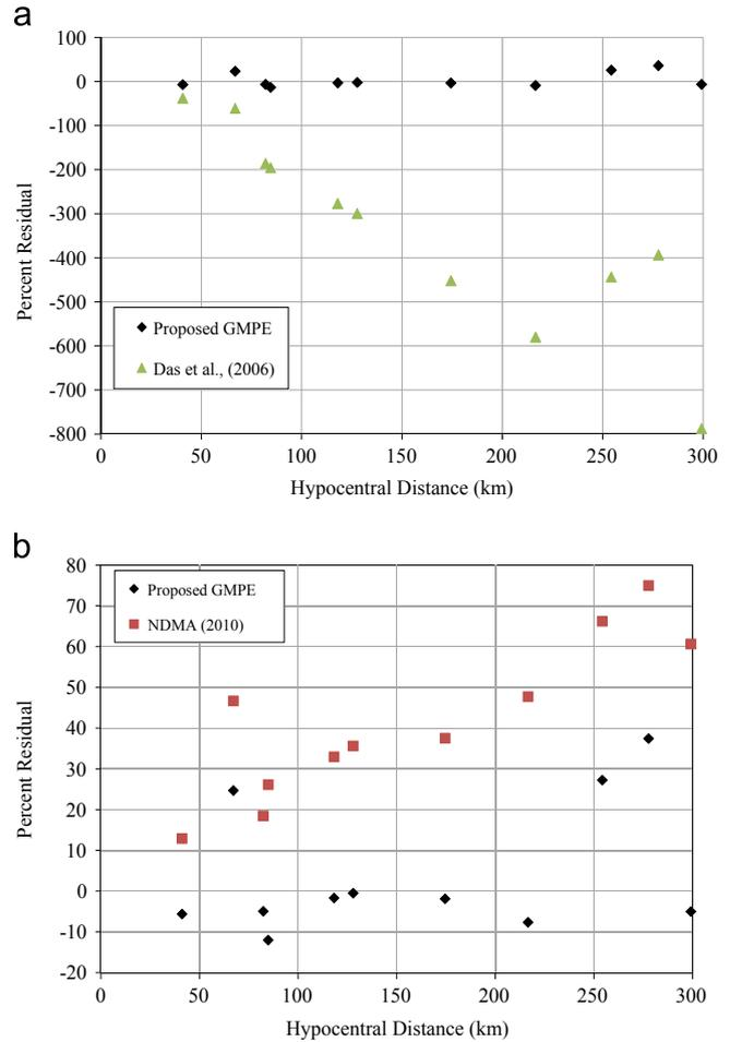
Fig. 16. (a) Plot of percent residual between recorded PGA and predicted PGA from Das et al. [23] and newly proposed GMPE for 2011 Nepal–India Border EQ. (b) Plot of percent residual between recorded PGA and predicted PGA from NDMA [54] and newly proposed GMPE for 2011 Nepal–India Border EQ.
