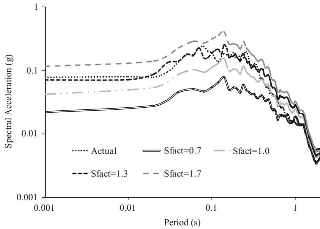
Fig. 5. Parametric study to establish the  $S_{fact}$  value in simulation for 1988 Manipur earthquake recorded at Harenjao.
