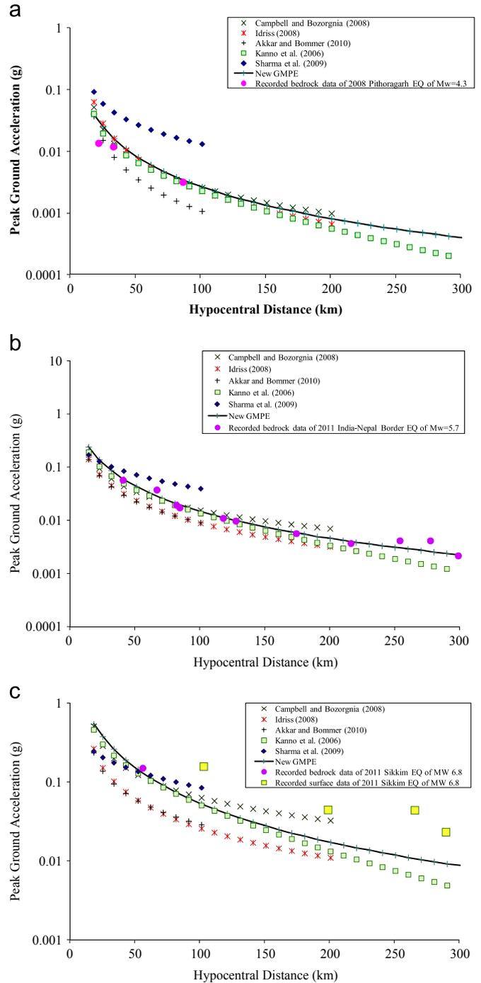
**Fig. 13.** (a) Comparison of new GMPE with first five highly ranked GMPEs and with recorded earthquake data for 2008 Pithoragarh earthquake of 4.3 in Mw. (b) Comparison of new GMPE with first five highly ranked GMPEs and recorded earthquake data for 2011 Nepal–India Border EQ with Mw of 5.7. (c) Comparison of new GMPE with first five highly ranked GMPEs and recorded earthquake data for 2011 Sikkim EQ with Mw of 6.8.
