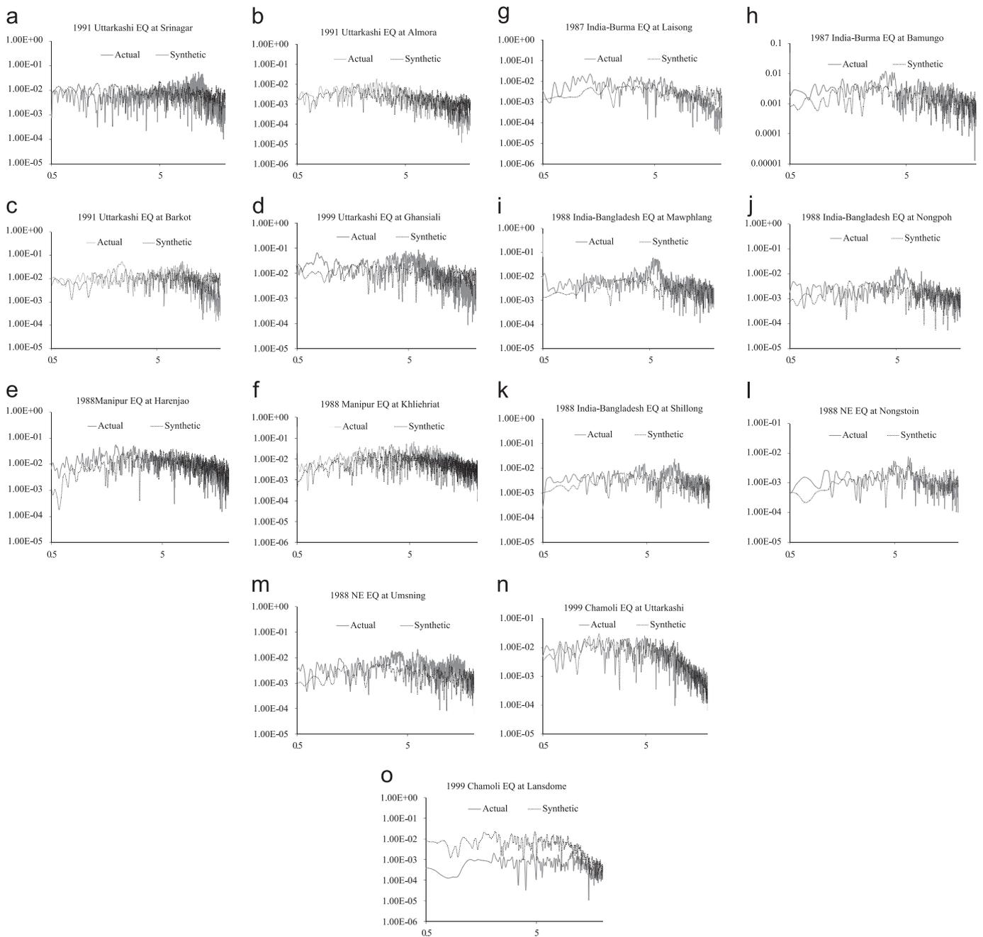
Fig. 9. (a–o) Comparison of Fourier amplitude spectrum for selected recorded and simulated ground motions.
