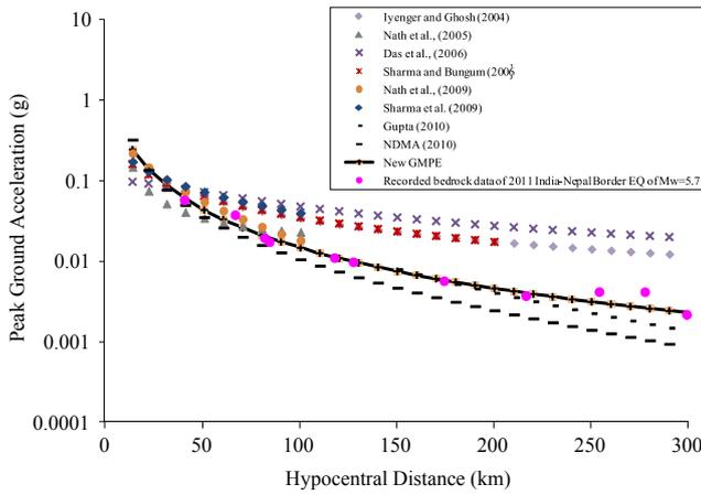
Fig. 15. Comparison of PGA predicted by various GMPEs with the recorded PGA during 2011 Nepal–India earthquake.
