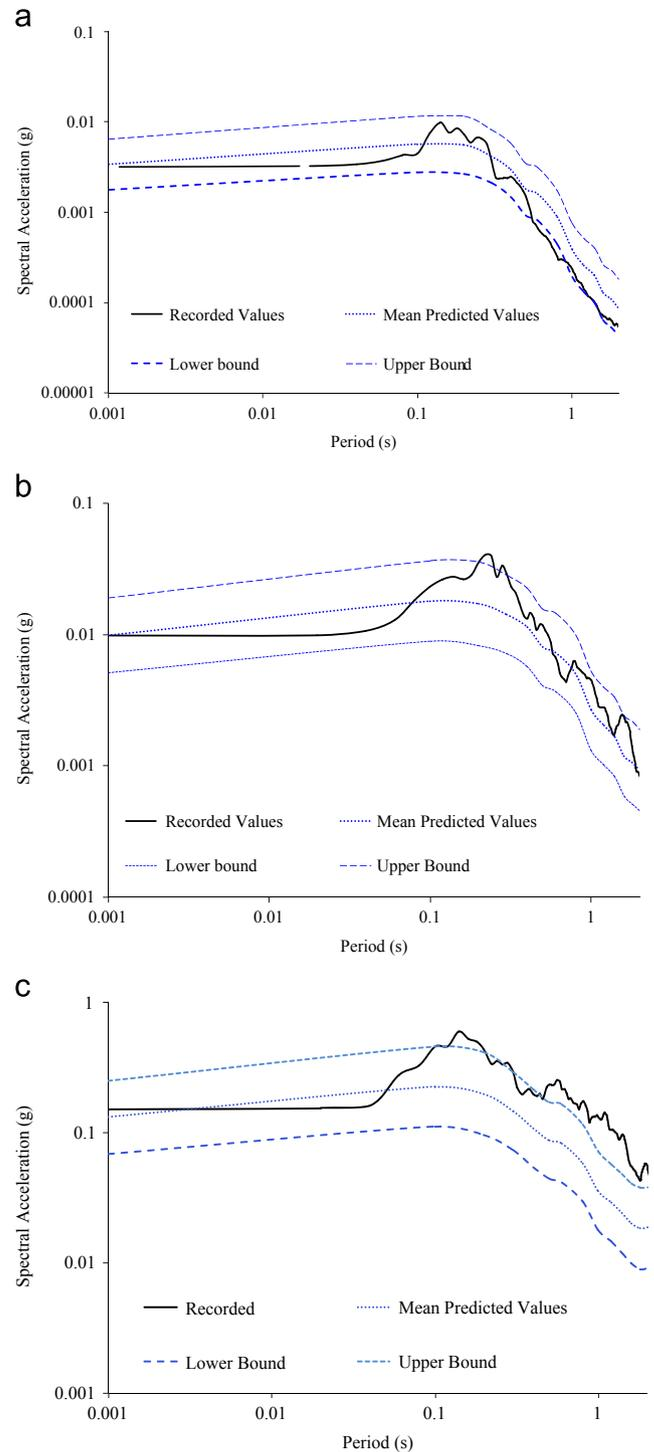
**Fig. 14.** (a) Comparison between proposed response spectrum in this study and response spectrum from the recorded 2008 Pithoragarh EQ at Champawat. (b) Comparison between proposed response spectrum in this study and response spectrum from the recorded 2011 Nepal–India Border EQ at Almora. (c) Comparison between proposed response spectrum in this study and response spectrum from the recorded 2011 Sikkim EQ at Gangtok.
