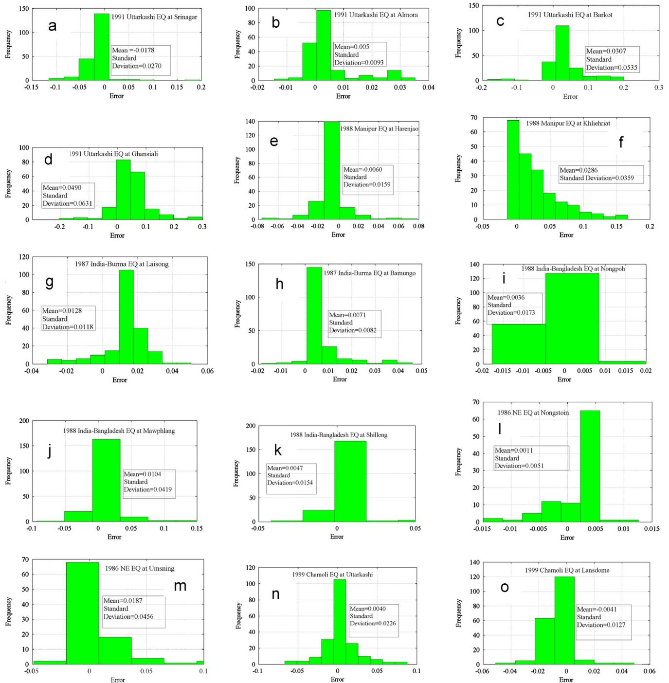
Fig. 8. (a–o) Error versus frequency plot for the response spectra shown in Fig. 6.
