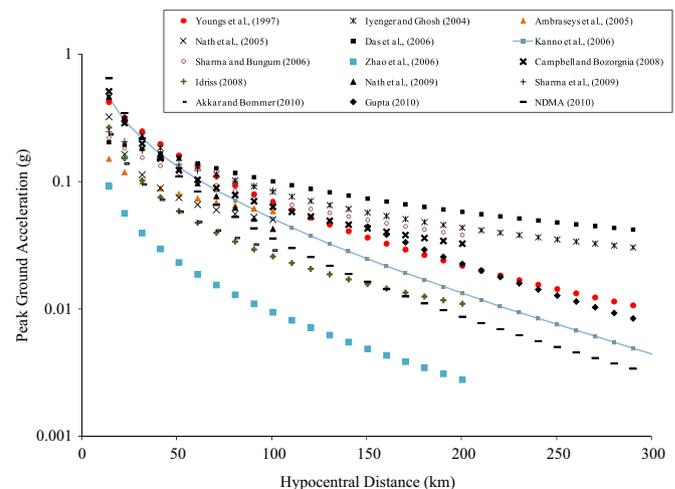
Fig. 1. Comparison of ground motion prediction equations applicable to Himalayan region for earthquake moment magnitude of 6.8.
