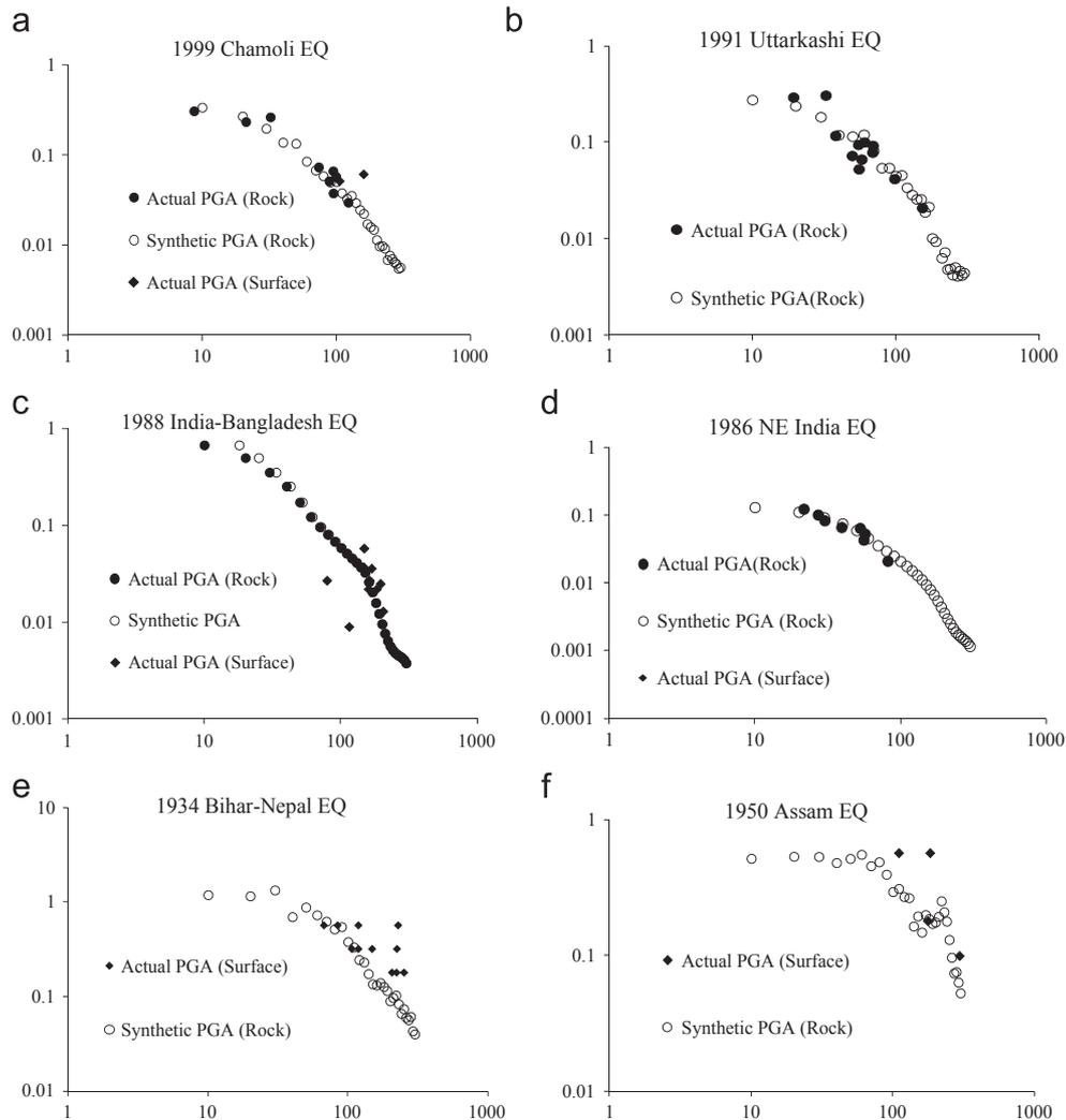
Fig. 12. (a–f) Comparison of simulated peak ground acceleration with recorded values at soil surface and rock level for selected earthquakes.
