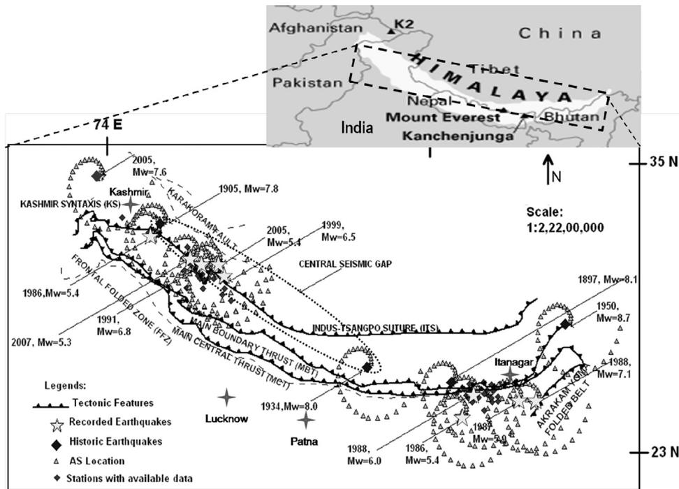
**Fig. 3.** Himalayan region with significant earthquake considered in this study along with Central Seismic gap and locations of ground motions used for attenuation relation (Modified after [40]).
