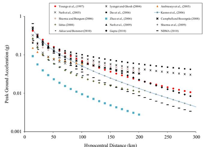
Fig. 1. Comparison of ground motion prediction equations applicable to Himalayan region for earthquake moment magnitude of 6.8.
