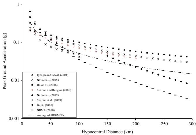
**Fig. 2.** Comparison of region specific ground motion prediction equations with the average of first five high ranked ground motion prediction equations (HRGMPEs) for an earthquake moment magnitude of 6.8.
