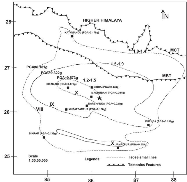
Fig. 11. Iseismal map in MMI with converted peak ground acceleration (left in counter) for 1934 Bihar–Nepal earthquake along with ground motion simulated locations and respective PGA.
