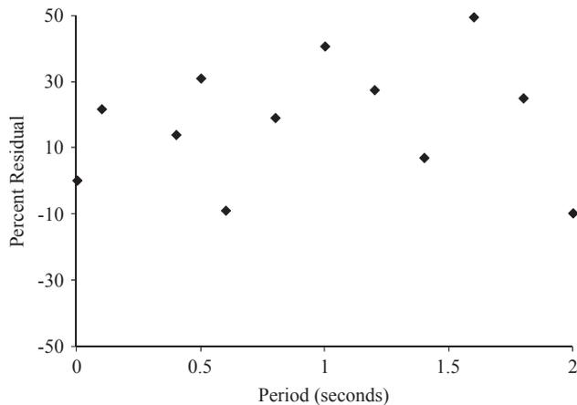
Fig. 17. Plot of percent residual between response spectra based on recorded data and newly proposed GMPE for 2011 Nepal–India Border EQ.
