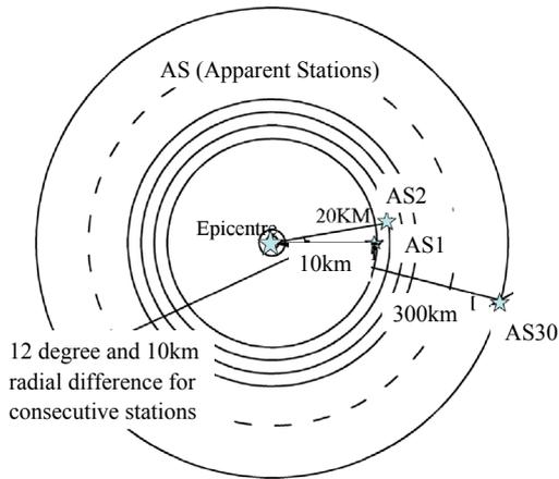
Fig. 10. Details of apparent stations distribution around the epicentre.
