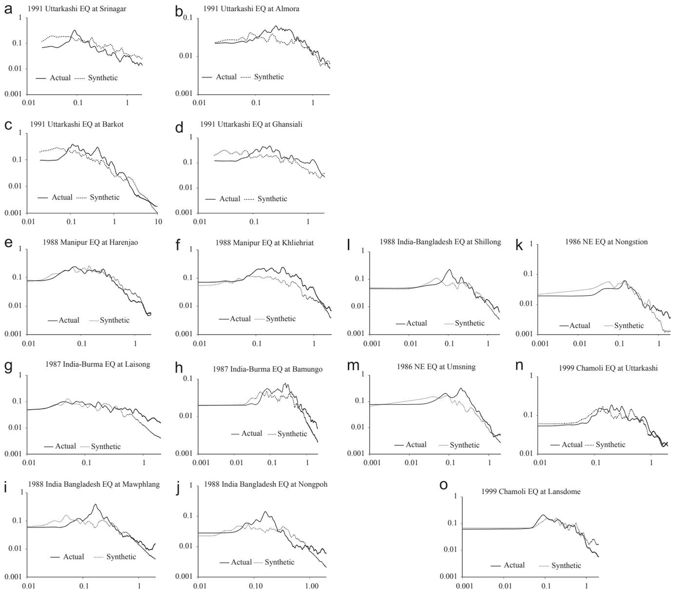
Fig. 7. (a–o) Comparison of response spectrum from recorded and simulated ground motions.
